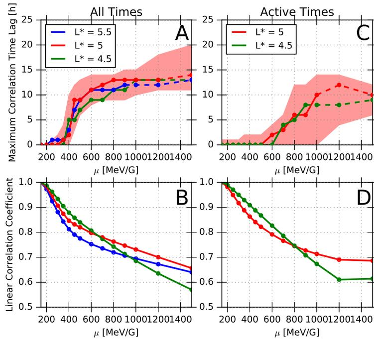
**Figure 2.** Results of the cross correlation analysis. Panels A and B show results with all 26 months of available data, panels C and D only includes results from within 5 days of a core enhancement event. Panels A and C show the time-lag that gives the maximum correlation coefficient with respect to the  $\mu = 100$  MeV/G population as function of  $\mu$  for 3 different  $L^*$  values. Panels B and D show the correlation coefficient as a function of  $\mu$ .
