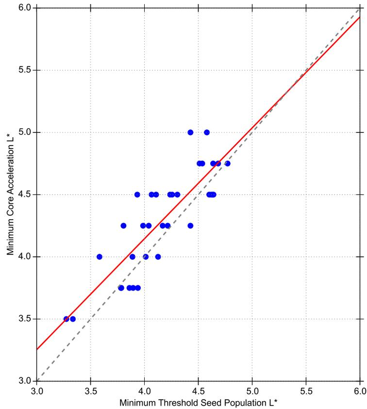
**Figure 6.** Relation between the minimum  $L^*$  where the seed population is above the threshold value and/or saturation limit of  $1 \times 10^{-4}$  and the minimum  $L^*$  where the core population was enhanced by at least a factor of 2. The red line is the best-fit line with a linear correlation of 0.84.
