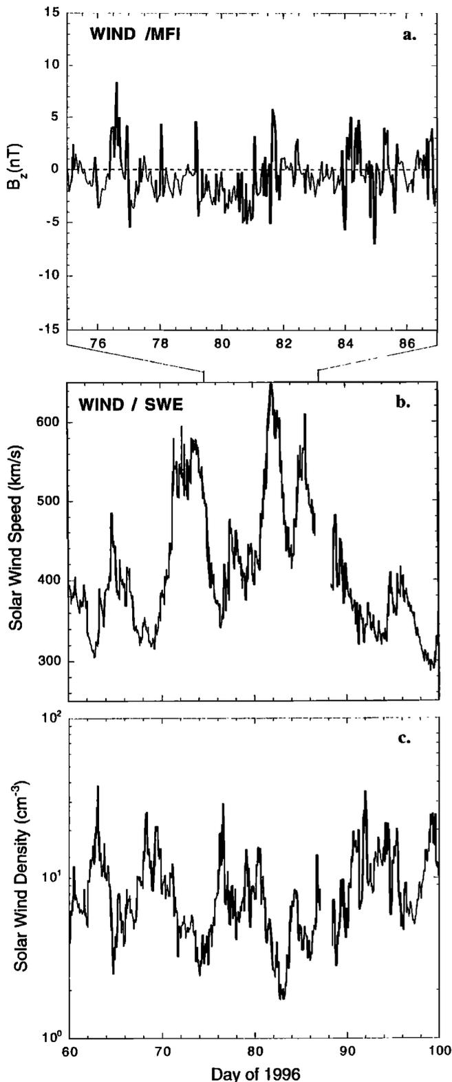
**Figure 3.** (a) Hourly averages of the interplanetary magnetic field  $B_z$  component for days 75-86. (b) Hourly averages of solar wind speed for days 60-100 of 1996. (c) Hourly averages of solar wind density for days 60-100 of 1996.
