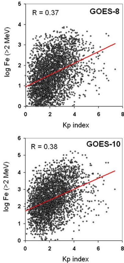
**Figure 1.** Correlation patterns for daily mean values of  $\log F_e$ , where  $F_e$  is the relativistic electron fluxes in counts/cm<sup>2</sup>·s·sr versus daily mean values of geomagnetic activity Kp index for Goes-8 and Goes-10 data for 1997–2002. The time delay of  $F_e$  with respect to solar wind speed and Kp index is 2 days. Trend lines and the Pearson correlation coefficients,  $R$ , are shown.
